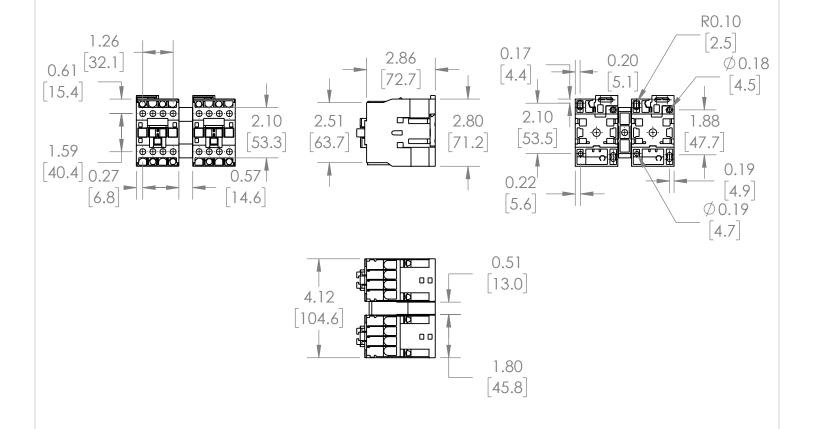
\*NOTE: BRAH ELECTRIC CONTACTOR BLC2D1810-Q6 IS AN AFTERMARKET DIRECT REPLACMENT FOR LC2D1810-Q6,LC2-D SERIES. SUITABLE FOR USE WITH LC2-D SERIES MOTOR CONTROL **SYSTEMS**
