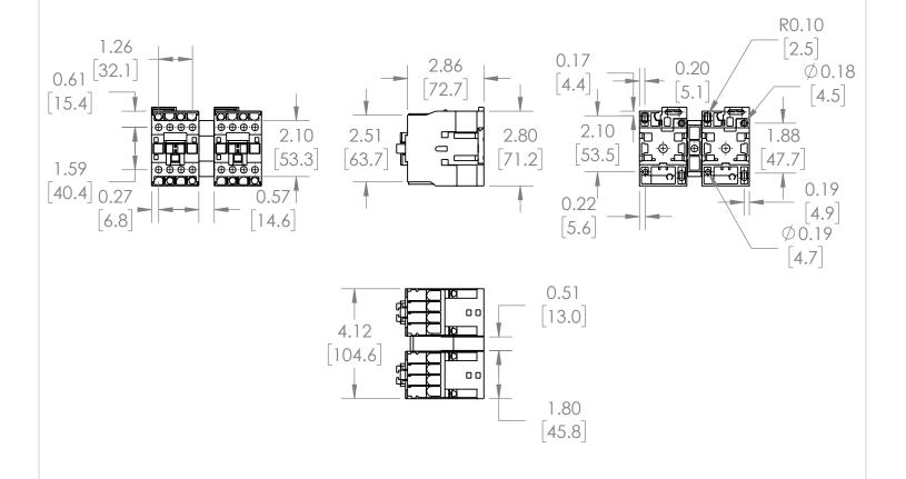
\*NOTE: BRAH ELECTRIC CONTACTOR BLC2D1810-T6 IS AN AFTERMARKET DIRECT REPLACMENT FOR LC2D1810-T6,LC2-D SERIES. SUITABLE FOR USE WITH LC2-D SERIES MOTOR CONTROL SYSTEMS
