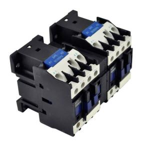
PART NUMBER – BLC2D3210-G6: BRAH Electric, aftermarket direct replacement contactors for Telemecanique LC2D3210-G6, TeSys D Series, type LC2D, 3P, 3PH, 50A, 600V, 10HP @ 240V, 20HP @ 480V, 30HP @ 600V, complete with 120V AC coil, 1 N/O auxiliary contact, AC magnetic contactor, suitable for use with LC2-D series motor control systems
