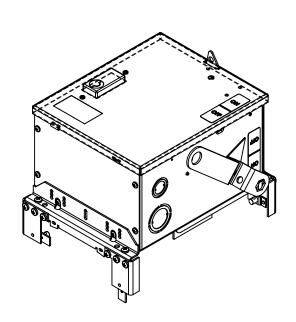
\* NOTE: BRAH Electric aftermarket AC362RI, aftermarket AC362RI, 60amp, 600volt, 3 phase, 3 wire, fusible style bus plug,includes weather stripping for drip protection, type BEC/AC, UL Listed assembly, complete with UL Recognized internal switch and components.
