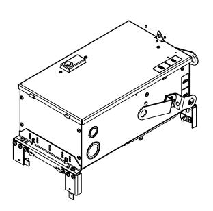
\* NOTE: BRAH Electric aftermarket AC423RG, 100amp, 240volt, 3 phase, 4 wire, with ground, fusible style bus plug, type BEC / AC, UL Listed assembly, complete with UL Recognized internal switch and components.
