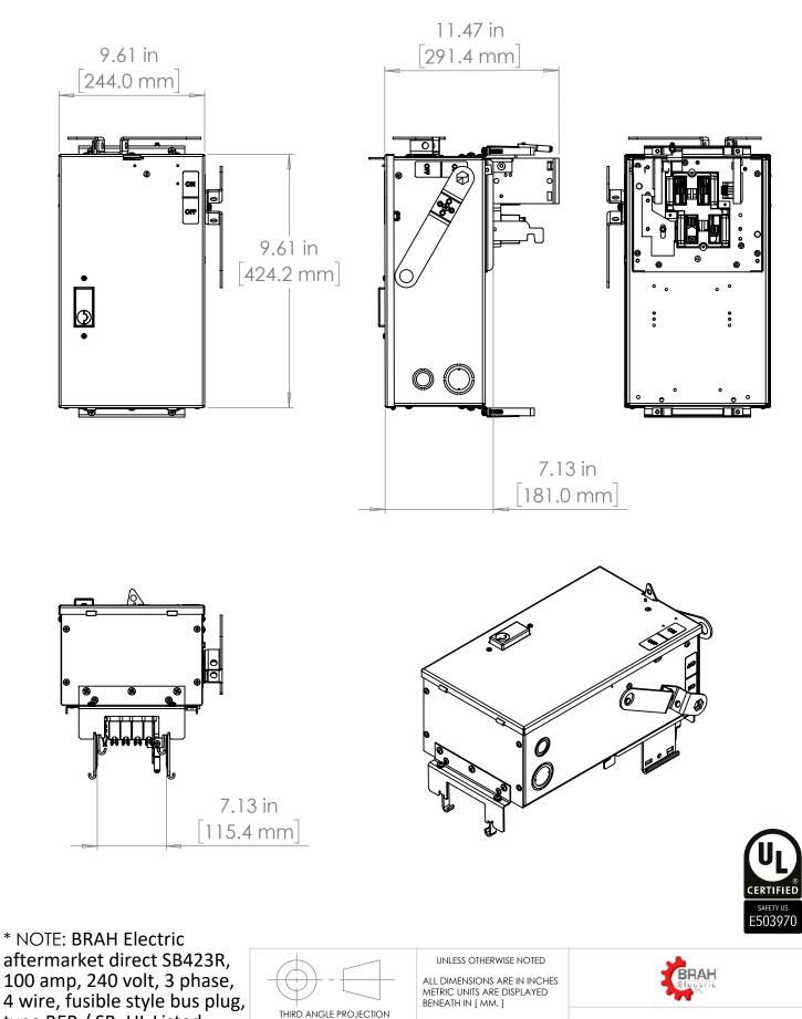
type BEB / SB, UL Listed assembly, complete with UL Recognized internal switch and components.
