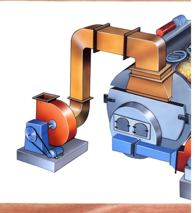
Three pass, smoke tube, she poiler for wood firing
