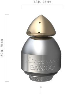
1/4 NPT, 1/4 BSPP, 9/16 MP, 3/8 MP The 2" Badger is a self-rotating swivel designed for cleaning 2–4 in. (51–102 mm) pipes with bends and long radius elbows, such as U-Tubes and process lines.
