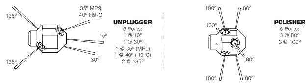
The correct head specification is based on the swivel, pressure, and flow of the pump.
