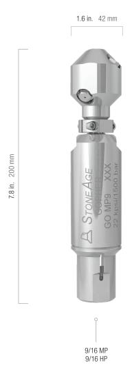
The Gopher self-rotary tool is ideal for cleaning evaporator tubes and liquor lines. It has the power to cut through coke, polymers, coatings and latex — anything clogging tubes or pipes as small as 2 inches (50 mm) in diameter. The Gopher is offered in two pressure ranges up to 40,000 psi (2800 bar).
