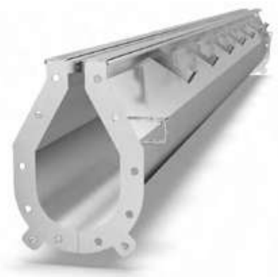
Figure 3: The 10,000 Series FoodSafe Slot Drain features 3/8" stainless steel embeds, welded to the drain and tied into rebar, creating a solid, unified drain-floor structure for long-term stability under
