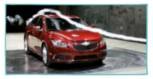
Moving cars encounter a force called air resistance. which slows them down. Air resistance increases with speed. If you double the speed of the moving vehicle, the air resistance quadruples.
