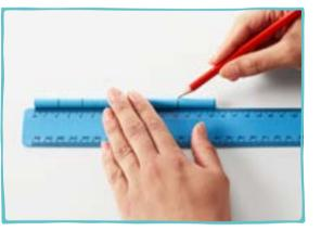
Draw lines on the tube at distances of 2, 4, and 12 cm ( $\frac{3}{4}$ , 1 $\frac{1}{2}$  and 5 in) from one end. These pieces will be your bearings.
