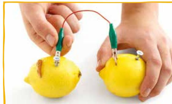
**3** Squeeze the clip on one wire so that it opens, like a crocodile's jaws. Place it around the screw in one lemon, so it grips it. Connect the other clip to the coin in another lemon.
