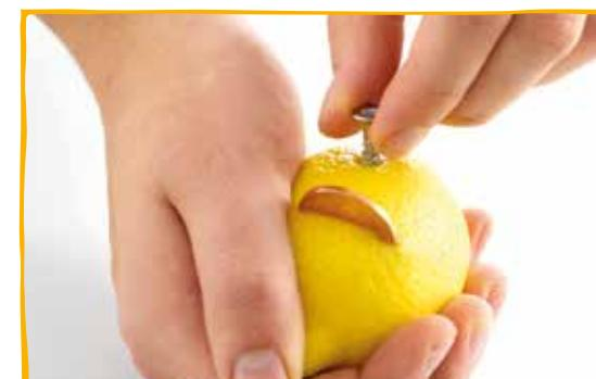
**2** About  $\frac{1}{2}$  in (1cm) from the center of the first lemon—on the other side to the coin—insert a galvanized screw. Twist it in, clockwise, to secure it in the lemon's flesh. Now repeat with the other four lemons, then arrange the lemons in a circle.
