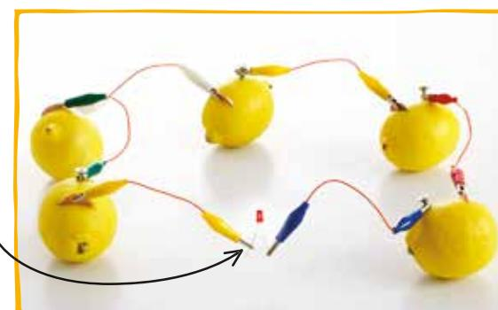
**5** Each LED has two legs, which are slightly different lengths. With the free end of the wire that is attached to the coin, fix the clip to the slightly longer leg of the LED.
