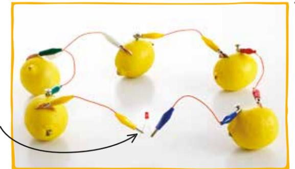
**6** Now connect the clip of the other free wire that is connected to the screw to the other, shorter leg of the LED. This now completes the circuit to make the LED light up.
