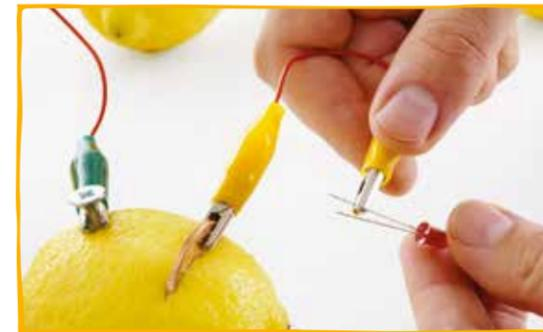
**5** Each LED has two legs, which are slightly different lengths. With the free end of the wire that is attached to the coin, fix the clip to the slightly longer leg of the LED.
