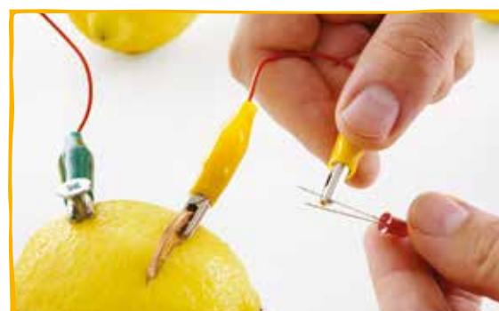
**4** Connect all the lemons—coin to screw—as in step 3. For the last lemon, attach a wire to its coin, but don't connect it to the screw in your first lemon. Instead, attach another wire to that screw.
