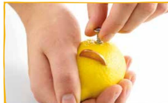
**2** About 1/2 in (1cm) from the center of the first lemon—on the other side to the coin—insert a galvanized screw. Twist it in, clockwise, to secure it in the lemon's flesh. Now repeat with the other four lemons, then arrange the lemons in a circle.
