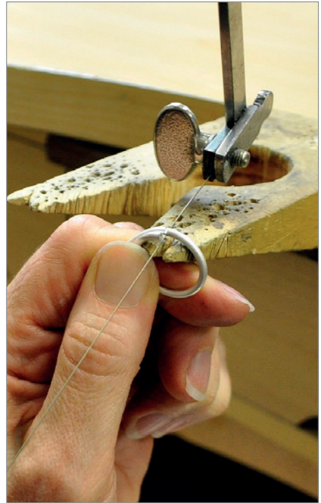
Sawing wire where it overlaps. (© Wug Laku)
