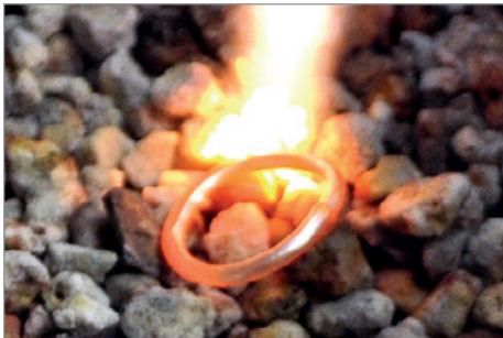
Keep an eye on the solder when using the torch on the silver ring. (© Wug Laku)
