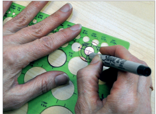
Use a circles template to mark bands on the copper discs. (© Wug Laku)
