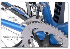
2 Thread one end of the new chain through the front derailleur (mech) cage until it catches on the teeth of the chainring. Turn the pedals and draw the chain downwards.
