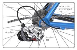
3 Pull the other end of the chain towards the rear derailleur so that it rests on the smallest cog of the cassette. It is now ready to be threaded through the rear derailleur.
