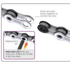
5 Bring the two ends of the chain together underneath the chainstay. Push the thin end of the replacement pin between the two links to hold the chain together.
