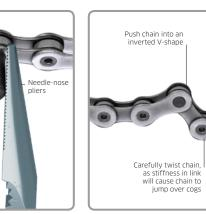
8 The chain will feel stiff at the join. Apply oil to the link and manipulate the chain with your hands until the link moves freely.
