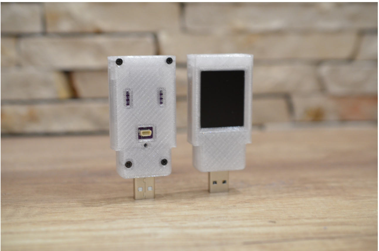
ESP32-DevKit12C-TFT with 1,8" 128x160pix TFT display (ST7735 driver)
