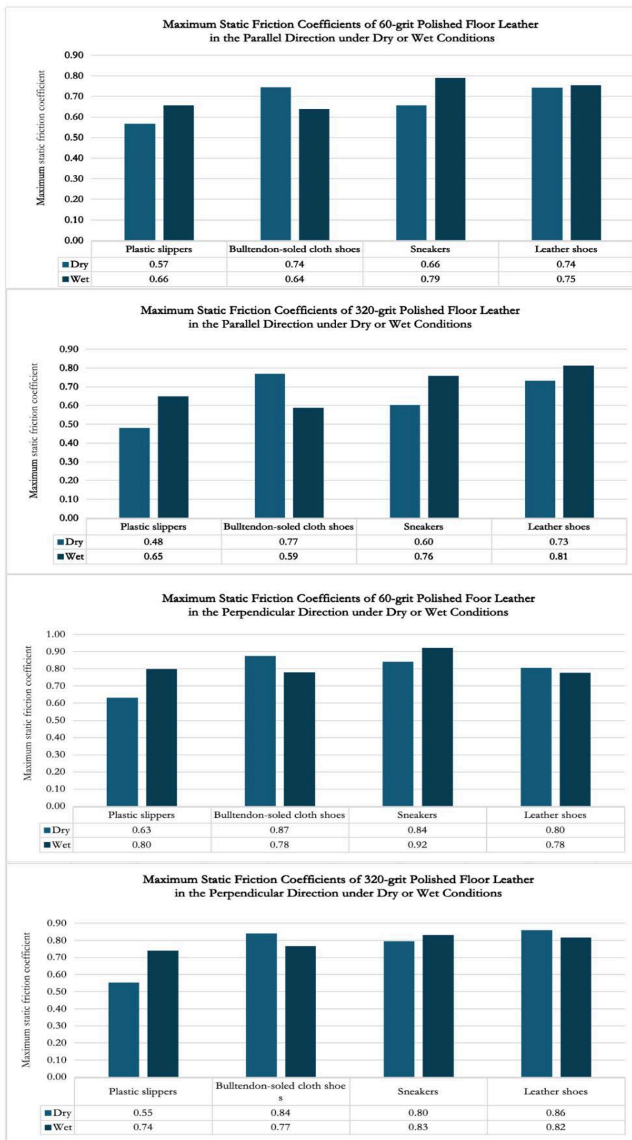
Figure 12: Maximum static friction coefficient under different rough surfaces and moisture conditions. Parallel/Perpendicular: Direction between abrasion marks and friction force.
