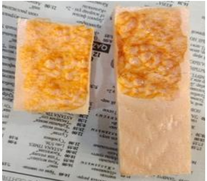
Figure 7: Unglued and Partially Dissolved Foam Plastic.
