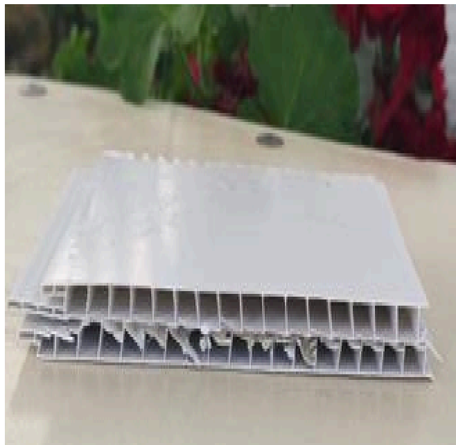
Figure 9: Glued Layers of Cellular Polypropylene.
