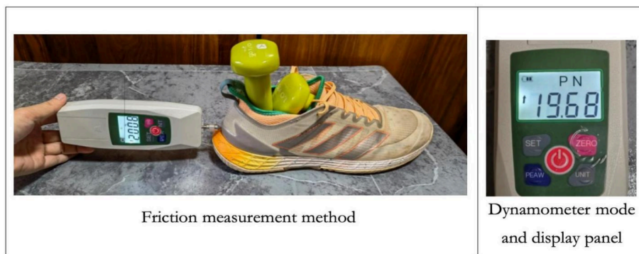
Figure 4: A visualization of the experimental setup for the friction test and tools used.
