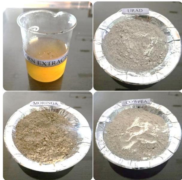
Figure 2: Four coagulants used for the coagulation. Corn Extract, Urad, Moringa Oleifera, and Cowpea.
