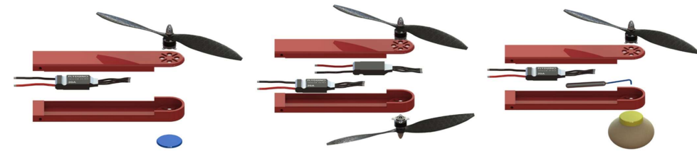
365 366 367 368 Figure 3: Types of rotor configurations in modular drones with avionic and electronic elements. Figure reproduced from 369 Brischetto et al. (1) Single-rotor configuration; (2) Double-rotor configuration; (3) Amphibious configuration.
