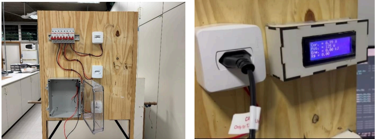
Figure 10: Image of the wooden panel and the power box (left), as well as the LCD display to display real-time readings (right). Source: Authora
