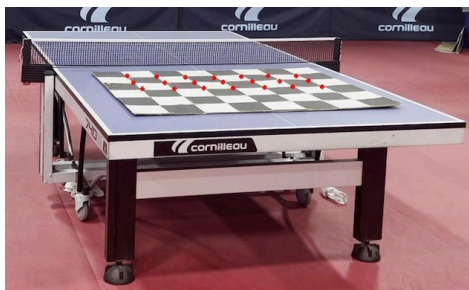
Figure 12. Reconstructed chessboard inner-corner through camera calibration and triangulation algorithms on camera 4 image.
