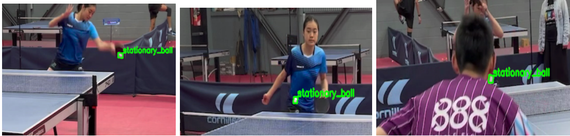
Figure 11: The images demonstrate success detections from images of clear view(left most), motion blur(middle), and partial occlusion(rightmost).
