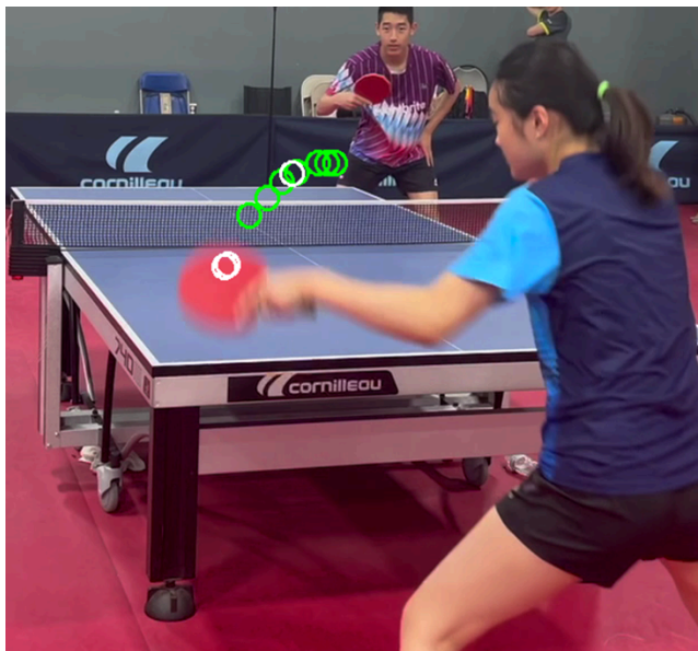
Figure 13. Tracked trajectory with ten balls, Kalman Filter predicted balls are in white circles. the detected balls are in green circles.
