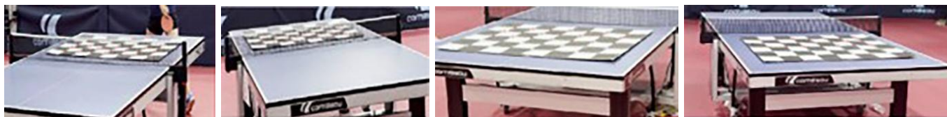
Figure 2: Hand-labeled inner corner of the chessboard from different cameras: camera 1 (leftmost), camera 2 (second-left), camera 3 (second-right), camera 4 (rightmost).
