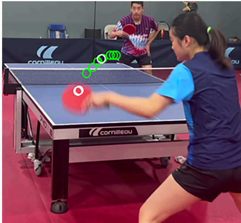
Figure 14: Tracked trajectory with ten balls, Kalman Filter-predicted balls are in white circles, the detected balls are in green circles.
