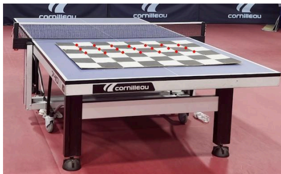
Figure 13: Reconstructed chessboard inner corner through camera calibration and triangulation algorithms on camera 4 image.
