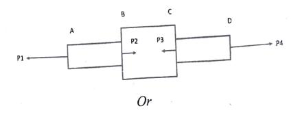
A rod consists of two parts that are made of steel and copper as shown in figure below. The elastic modulus and coefficient of thermal expansion for steel are 200 GPa and  $11.7 \times 10^{-6}$  per °C respectively and for copper 70 GPa and  $21.6 \times 10^{-6}$  per °C respectively. If the temperature of the rod is raised by 50°C, determine the forces and stresses acting on the rod.
