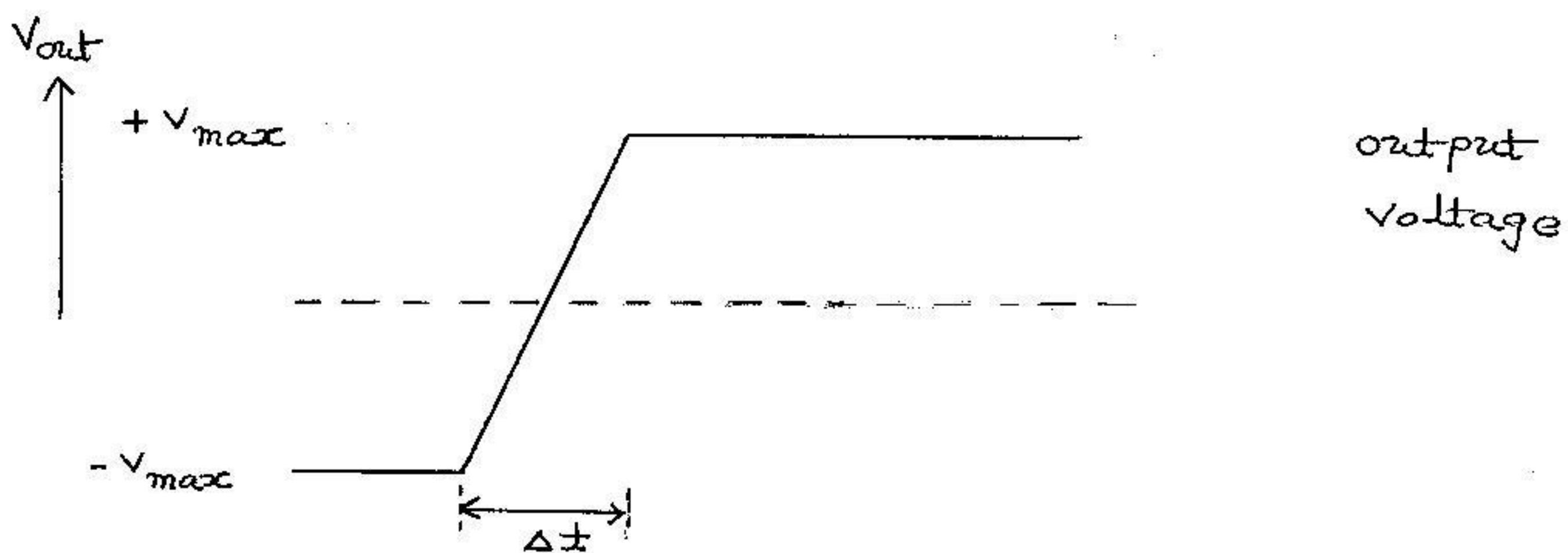
A certain time interval  $\Delta t$ , is required for the output voltage to go from  $-V_{max}$  to  $+V_{max}$  when step input is applied.
