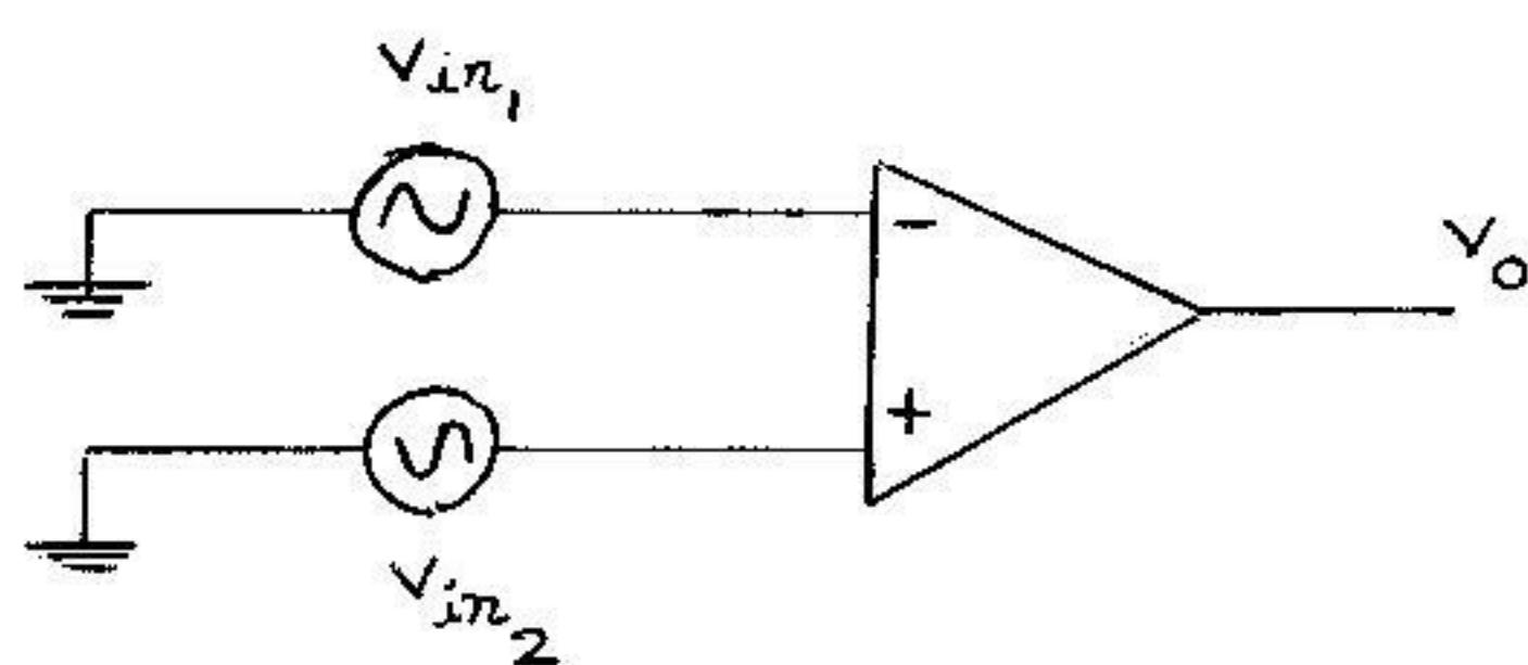
In common mode, the two signal voltages of same phase, frequency and magnitude are applied to the two inputs as shown in the figure below.
