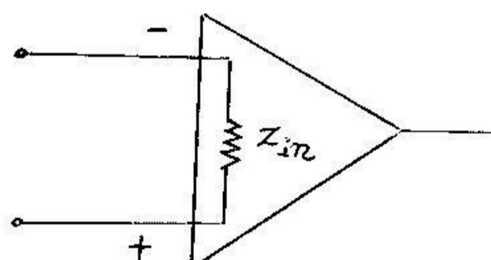
The input impedance in differential mode is obtained by the ratio of change in the differential input voltage and change in the bias current.
