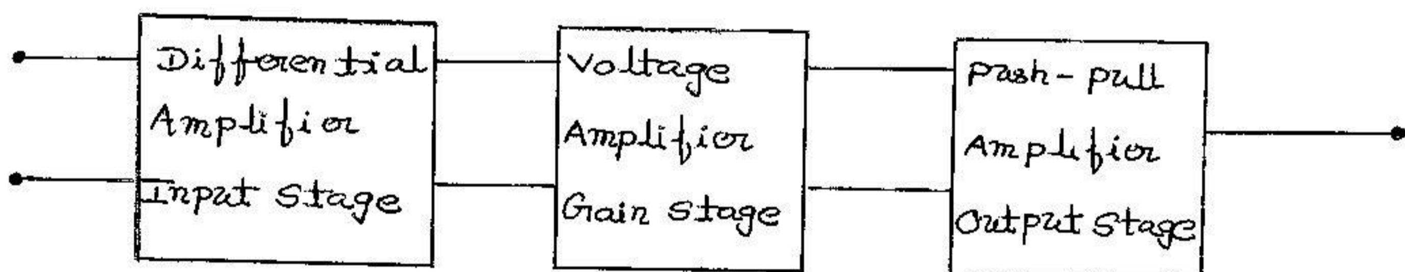
A typical op-amp contains the following three stages:
