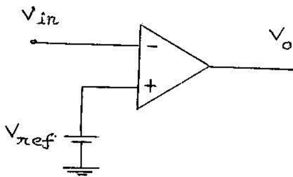
Figure shows the circuit diagram of an inverting comparator with the reference voltage  $V_{ref}$  applied at the noninverting input. The input signal is applied at the inverting input.
