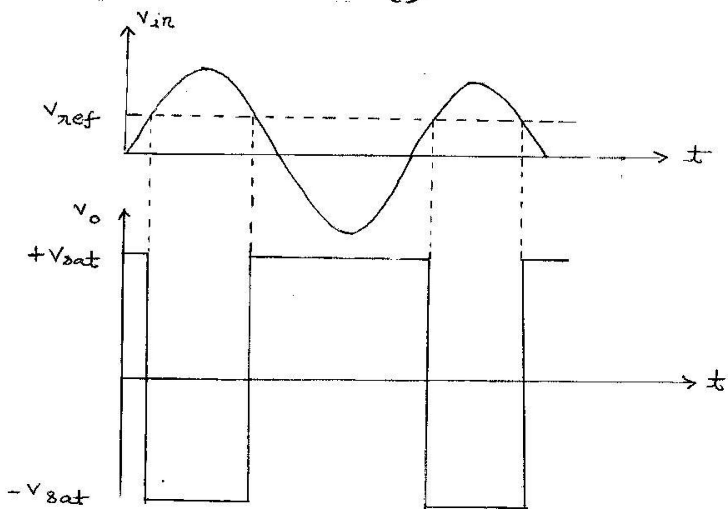
When  $V_{ref}$  is set to zero, the comparator is called Zero crossing detector. The input and output waveforms are shown below.
