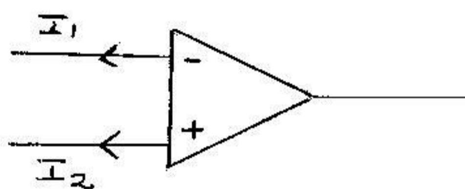
5. Input Impedance :- The input impedance in the differential mode is the total resistance between the inverting and the non inverting inputs as shown below:
