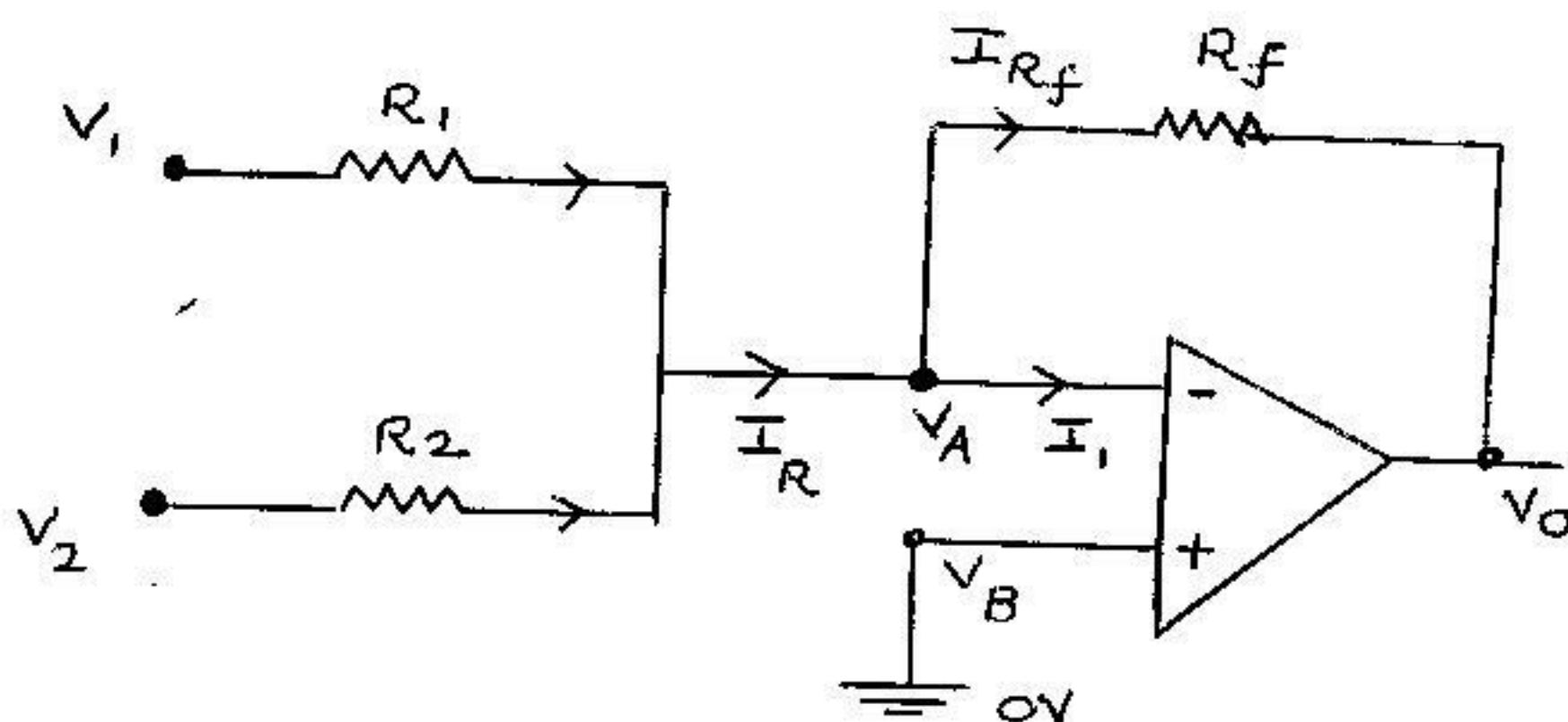
Figure above shows the circuit diagram of an inverting adder. By the concept of virtual ground we have
