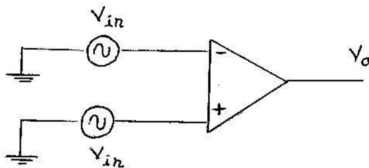
When equal input signals are applied to both inputs, they tend to cancel resulting in a zero output voltage. This action is called common mode rejection.
