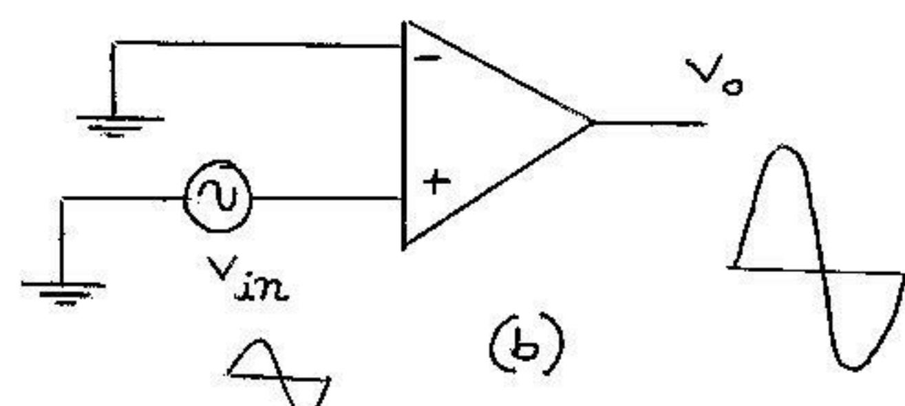
In the case when the signal voltage is applied to the inverting input as in figure (a), an inverted amplified signal voltage appears at the output. In case, when the signal voltage is applied to the non inverting input as in figure (b), a non inverted amplified signal voltage appears at the output.
