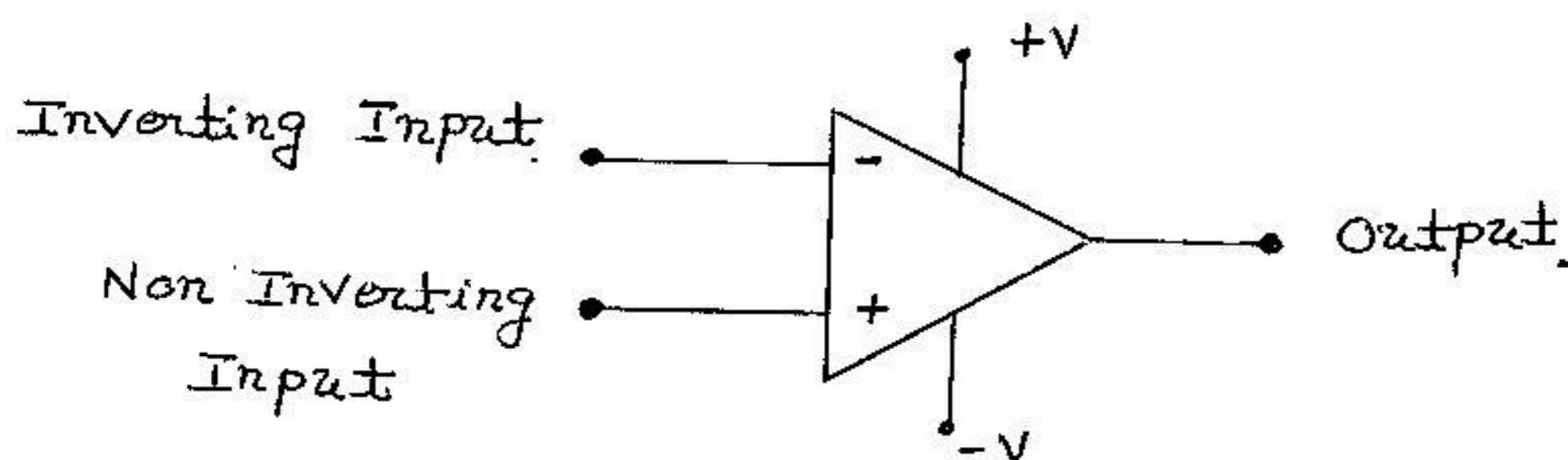
Figure above shows the circuit symbol of op-amp. It has two input terminals, the inverting input and the non inverting input, and one output terminal. Most op-amps work with two dc supply voltages, one positive and the other negative as shown in the figure.
