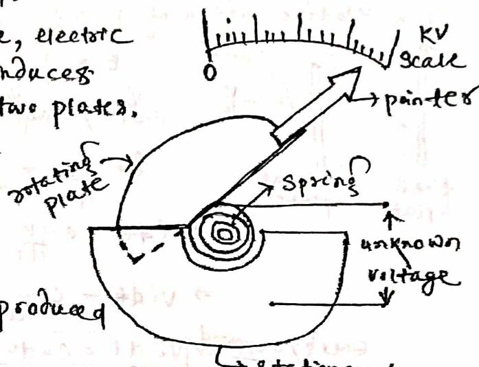
Adv :- → give correct measurement in both ac & dc.
