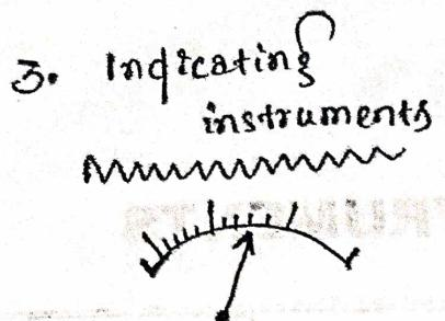
→ indicates the magnitude total amount of an electrical quantity at the time when it is being measured, given by a pointer.
