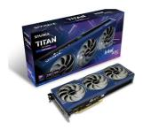
The SPARKLE Intel Arc B580 TITAN OC provides performance and versatility for gamers and creators alike. Featuring graphics capabilities, this card supports a maximum external resolution of  $7680 \times 4320$  at 120 Hz through its HDMI and DisplayPort interfaces. With 12 GB of GDDR6 SDRAM and a 192-bit bus width, bandwidth reaches 456 GBps, facilitating smooth gameplay.
