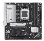
The ASUS PRIME B850M-A WIFI motherboard is designed to deliver performance for the modern user. Featuring support for AMD Ryzen processors, this micro ATX motherboard includes multiple expansion slots such as PCIe 5.0 x16 and PCIe 4.0 x16, ensuring connectivity for high-performance components. The motherboard supports DDR5 SDRAM with speeds reaching up to 4000 MHz, allowing for efficient multitasking and improved system responsiveness.
