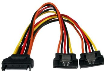
Add an extra SATA power outlet to your PC Power Supply. The PYO2LSATA 6" SATA Power Splitter Cable features a SATA 15-pin plug that connects to a single computer power supply SATA connector and breaks out into two latching SATA 15-pin receptacles, which enables you to connect two Serial ATA drives to a single SATA power connection on the computer power supply.
