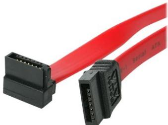
Make a right-angled connection to your SATA drive, for installation in tight spaces. The SATA12RA1 Right Angle (90-degree) SATA Cable features a standard (straight) SATA receptacle as well as a right-angled SATA receptacle, providing a simple 12-inch connection to a Serial ATA drive, with full SATA 3.0 bandwidth support of up to 6Gbps when used with SATA 3.0 compliant drives.
