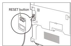
3. Press the TEST button lightly with a sharp edge such as a pen tip. The depressed RESET button will stick out again. This is the end of the check procedure.
