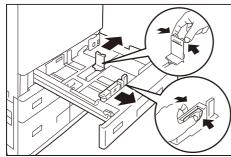
Fan a stack of paper, face the print surface up, and then load the paper with edges aligned according to the direction of the arrow.
