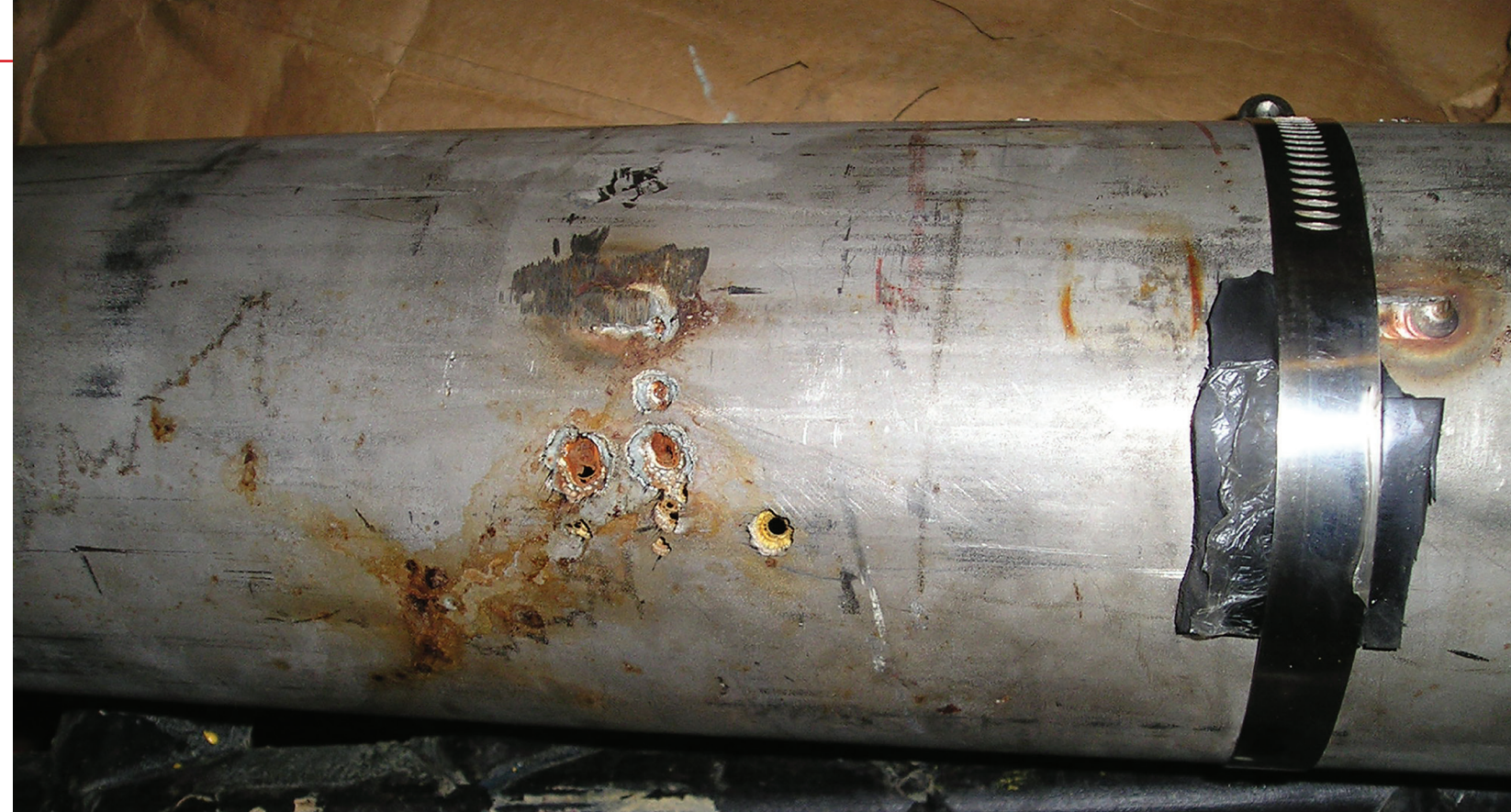
Pictured: Failing pipes with holes that caused leaks.
