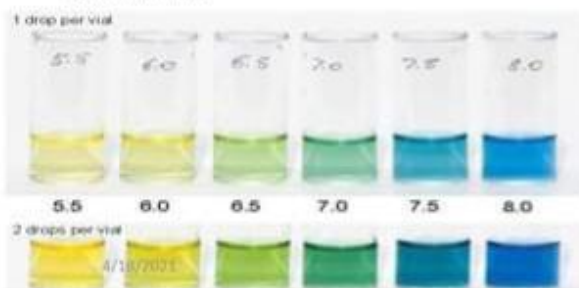
Bromothymol Blue pH Tester pH Color Chart
