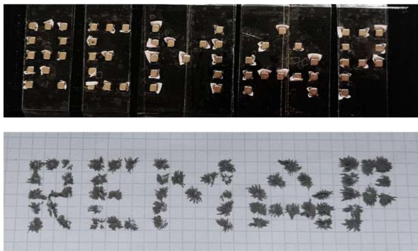
Figure 3: Demonstration of the reusable magnetic patterning, or "magnetic writing," at a distance using the action of magnets on iron powder.
