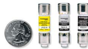
LP-CC, FRQ-R, KTK-R — Class CC, 600 V, 200 kA IR up to 30 A
