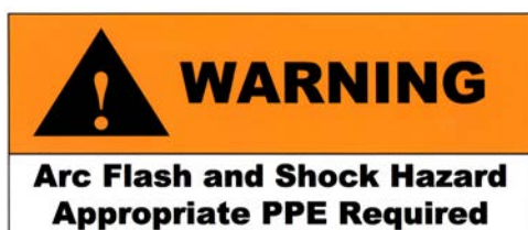
Figure 6.4.4.a Label complying with NEC 110.16(A)
