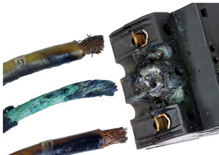
Figure 7.7.7.a This disconnect's middle, lineside conductor became loose and created an excessive thermal condition that damaged the terminal, along with the middle and the adjacent conductors.
