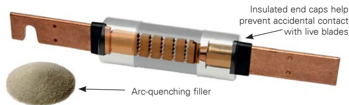
Figure 3.1.3.2.a Typical Class R Low-Peak fuse.
