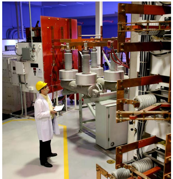
The Eaton Bussmann Division's Paul P. Gubany Center for High Power Technology is the electrical industry's most comprehensive facility for testing and certifying device and equipment SCCRs. Capable of performing electrical tests up to 600 V three-phase, 300 kA fault current for meeting ANCE, ANSI, CE, CSA, ETL, IEC and UL testing requirements.
