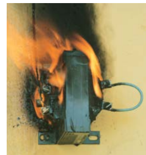
Figure 3.1.4.2.b Fires can result if the correct OCPD amp rating is not applied.
