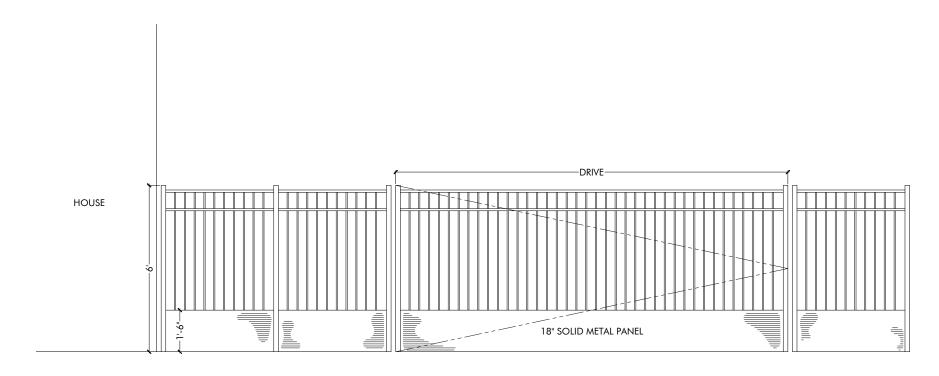
\*FIELD VERIFY DIMENSION OF POSTS AND SLOPE OF DRIVE TO INSURE GATE DOES NOT DRAG ON PAVEMENT AND MAINTAINS 2" OR LESS GAP AT BOTTOM TO PREVENT DOG ESCAPE.
