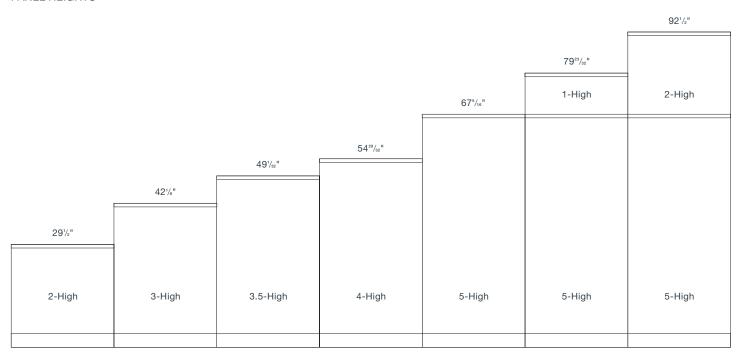
Xsite frames are available in five different base heights and can be built up to 80" and 93" tall by adding one or two stackers. Frames can be extended in three-inch increments so offices can be sized as needed.
