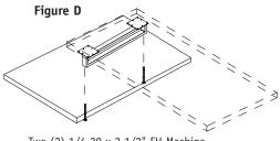
Two (2) 1/4-20 x 2 1/2" FH Machine Screws
