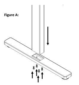
Partially screw four of the provided M8 x 16 screws into the holes on both 2 legs as shown in Figure B.
