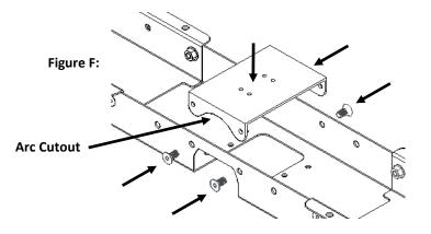
Note: Verify that the motor mount plate is oriented the same as in Figure G. The arc cutout must be facing away from the user.
