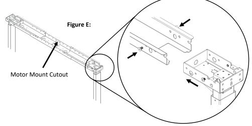
Attach the adjustable upper channel (Set to the correct length) to both legs
