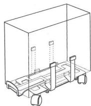
**Step 2:** Place CPU into unit. The arms will automatically close to secure the CPU in place.
