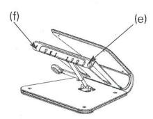
3. Pull out Height Adjustment Pin (b) to change viewing height of notebook screen. Release at desired height.
