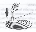
**CAUTION!** Use only a quad tube compact 26W fluorescent bulb with Base Type: G24Q-3. Always unplug the Task Light before attempting to remove or install bulb.
