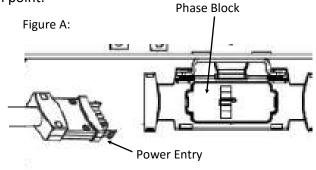
Using the supplied self drilling screw, secure the loop clamp and power entry whip to the bottom side of the powered beam. Be sure to place the screw in either the right of left side groove (Figure B). Clamp may be placed anywhere along beam within 6 inches of an open connection where power infeed is needed.
