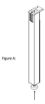
Determine where along the center beam you would like the power entry. Using the four provided screws attach the top mounting plate to the bottom side of the center beam as shown in **Figure A**. Verify the power entry pole will not interfere with any other components before attaching.
