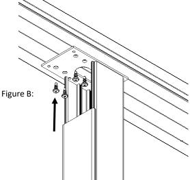
Remove the power entry pole cover to run power entry whip. Reattach cover when power has been connected.
