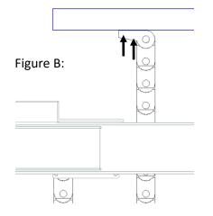
Verify chain runs up and down without binding or dragging. Run required electrical cords through the E Chain to prevent pulling and tangling.
