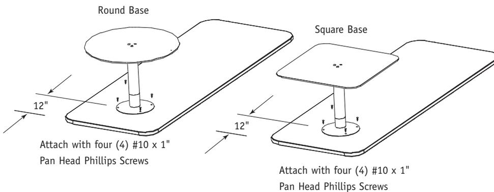
**Note:** If Square Base is used, adjust the height before attaching to the Worksurface. This will insure Square Base is aligned with the Worksurface.
