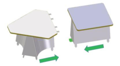
Align the prebored holes in bottom of the worksurface with the brackets.
