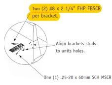
Lay all three panels onto the brackets. Align mitered corners and push in to remove any gaps between the shelf and the unit. Starting with the two end panels, use the screwdriver attach the shelf to the brackets. Finish by attaching the center panel.
