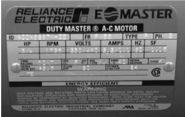
Figure 1: Typical label on an electric motor.
