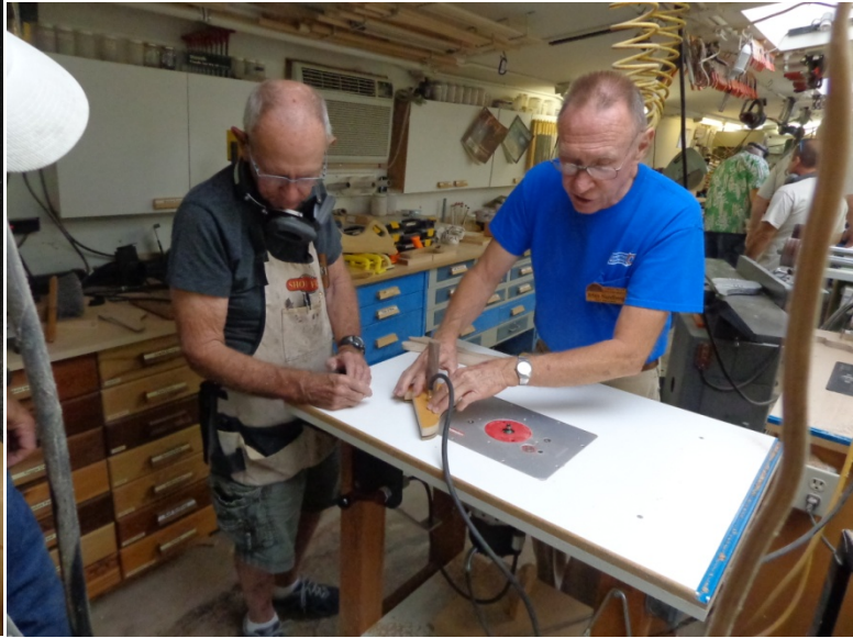
Arlen shows Richard K. how to cut fingers with a jig.
